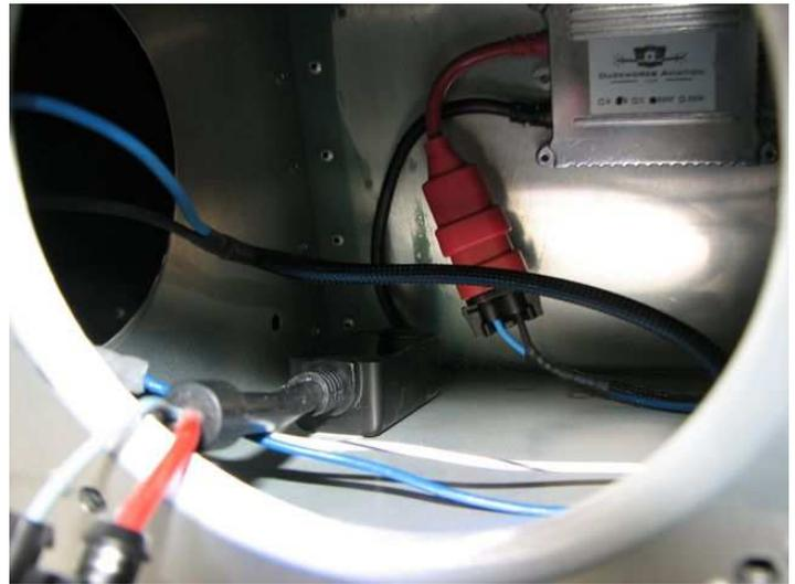
Connect the landing light wires to the HID module (Red or Blue is Pos, Black is Neg). Stick the module to the wing spar extension with a double sided pad.
